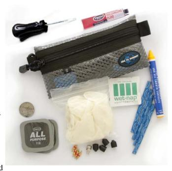
RIDER! Ultimate Tech Tire Repair Kit. It consists of several universal patches for tube and tubeless tires, some self vulcanizing rubber insertion strips (try to find these at the auto parts store) and even parts to repair faulty valve cores. Here a list of what's inside and why.
